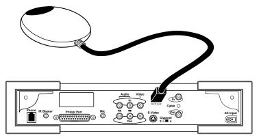
If you want to place the Internet Terminal in a cabinet, or somewhere out of view, use the webeye. Then, point the remote control at the webeye (not the Internet Terminal) in order to control the Internet Terminal.
